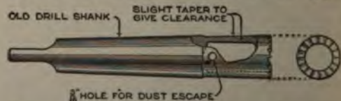
A Tool Made from the Shank of a Broken Twist Drill Provides a Ready Means of Cutting Out Small Wooden Plugs of a Given Diameter
